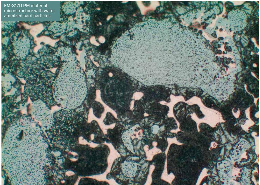
that make series production difficult, according to Denis Christopherson, Federal-Mogul Powertrain's valve seats and guides group director of R&D. "Higher alloying and the use of hard particles can potentially result in catastrophic failure of the cutting tool by notching, chipping or fracture, as the particles present an
