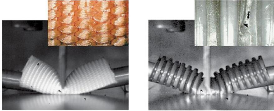
❶ Damage comparison of the CrushShield textile covering (left) versus a corrugated nylon tube (right) during and after the free-fall test
