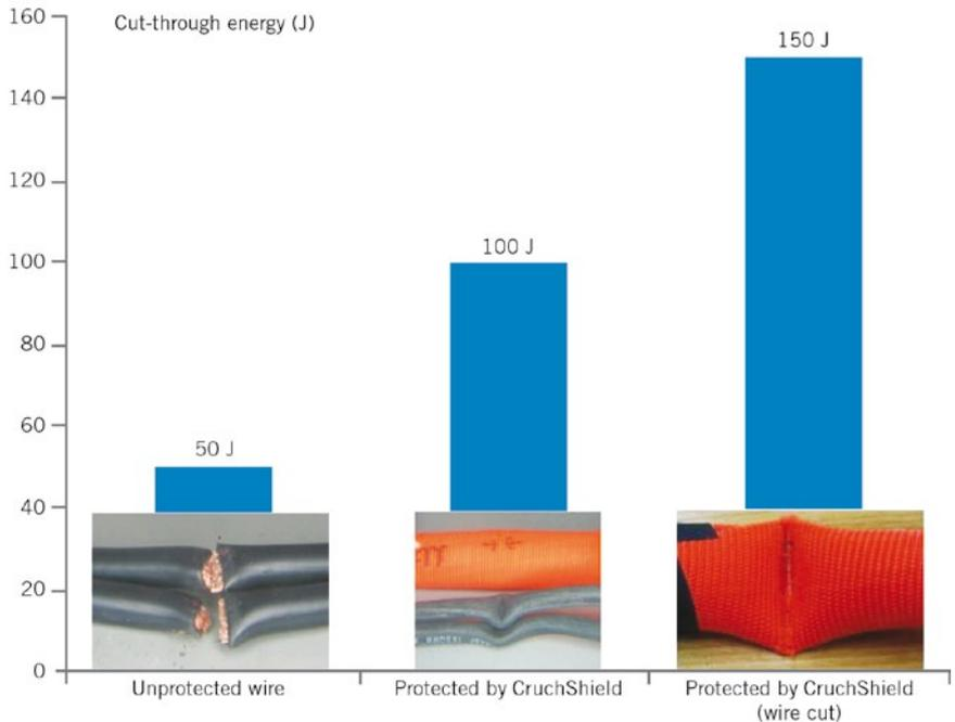
❷ Free-fall test results for the unprotected cable (left) as a baseline, and CrushShield (middle and right); on the right, the cable is damaged beneath the CrushShield, which remains intact and continuing to cover the high-voltage conductor
