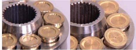
*High performing fluid protects the yellow piston shoes from erosion on this hydraulic pump. The brass piston shoes are completely scratch and erosion free.*
