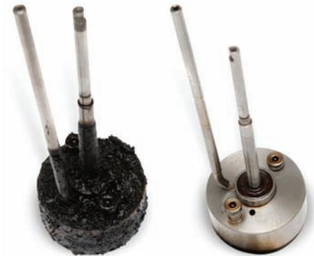
*A dramatic difference when comparing a housing with oxidation build-up and a clean part protected with quality tractor hydraulic fluid.*
